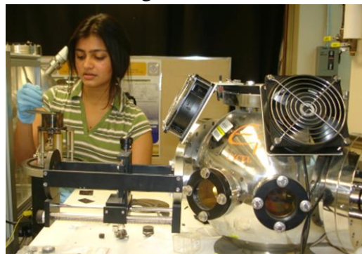
Figure 1. An REU student making a nanostructured sample using the PLD process
