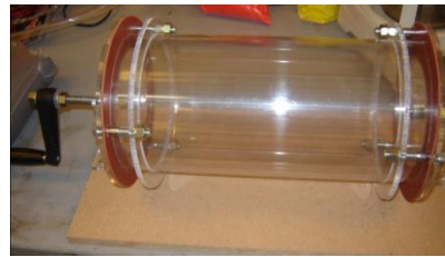
Figure 6: Tumbler apparatus for segregation demonstration
