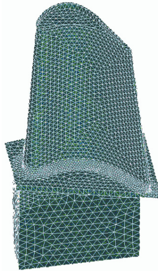
Fig. 6. FEA mesh for mechanical analysis
