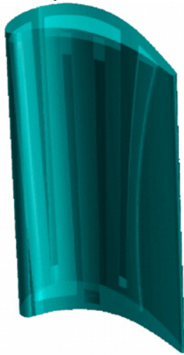
Fig. 5. Initial 3D solid body model of the rotor blade
