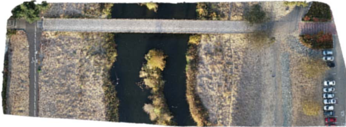
Figure 1. Map of the Calaveras River on the University of the Pacific campus created using 100 UAV images and five ground control points.
