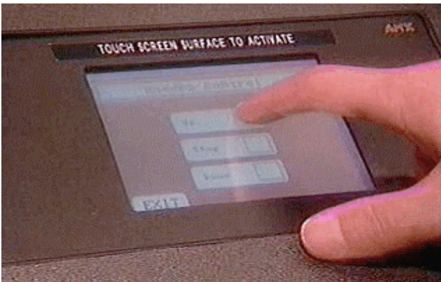
Figure 1. The AMX touch-screen interface, displaying the screen-control sub-menu of the hierarchical menu. In order to navigate to another function, the user must first press the EXIT button at the bottom left of the screen.
