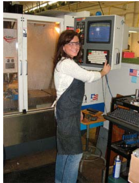
A student programs the Fadal CNC mill to fabricate wheels for the Moonbuggy.
