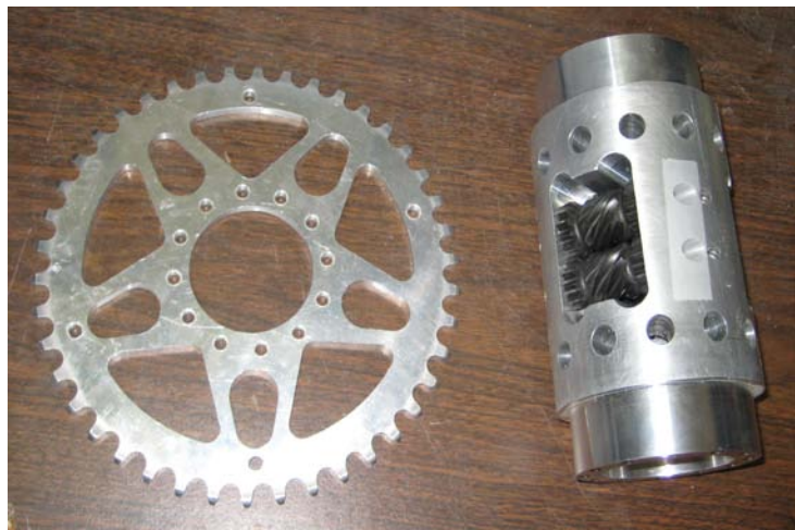
A custom-designed sprocket (left) and differential (right) created and manufactured by students on the Formula SAE team.
