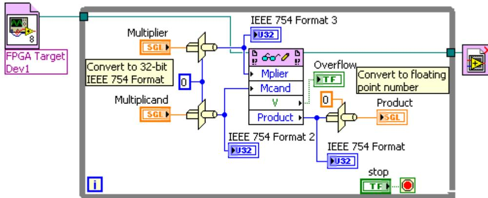
Figure 9. Floating-Point Multiplier Host VI.
