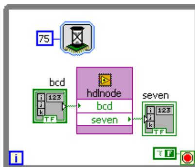
**Figure 4. LabVIEW FPGA Module HDLNODE.**
