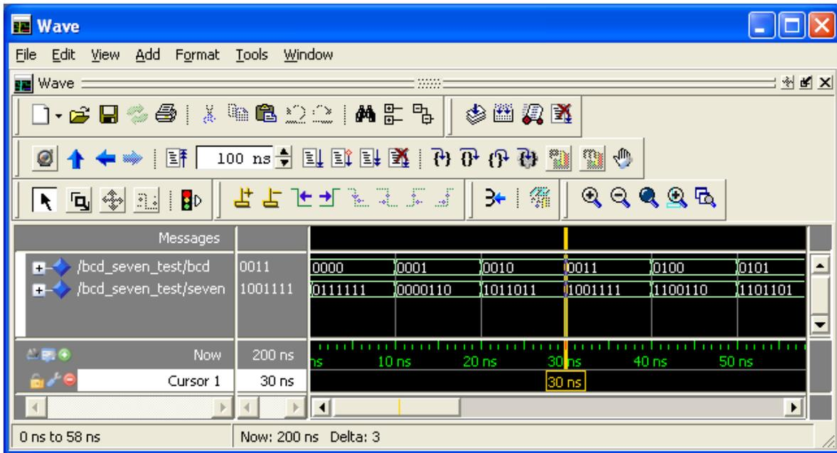
**Figure 3. VHDL Simulation Waveform.**
