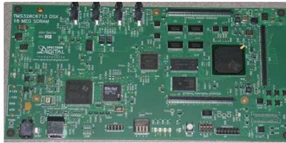
Figure 1. The TMS320C6713 DSK board.
