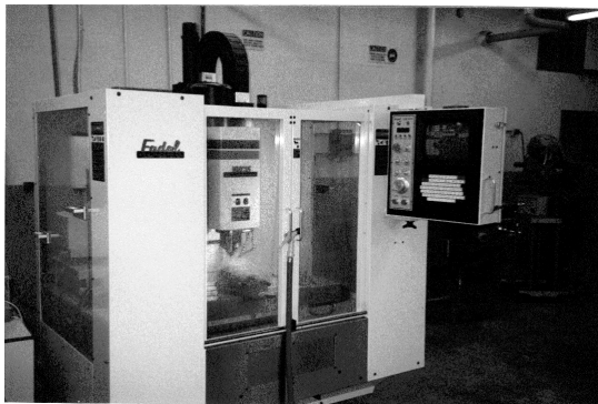
FIG. 2. Fadal VMC-15 Vertical Machining Center installed in the Integrated Laboratory for Manufacturing Education.
