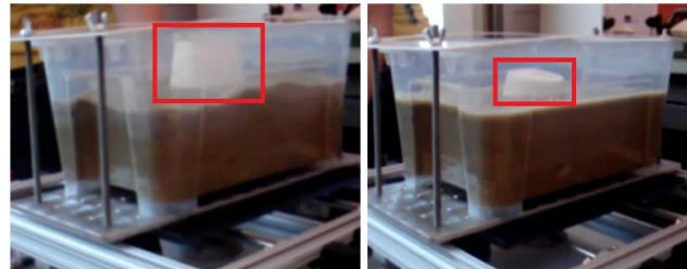
Figure 2. Soil Liquefaction Demonstration: Structure Before (Left) and After (Right) Shaking
