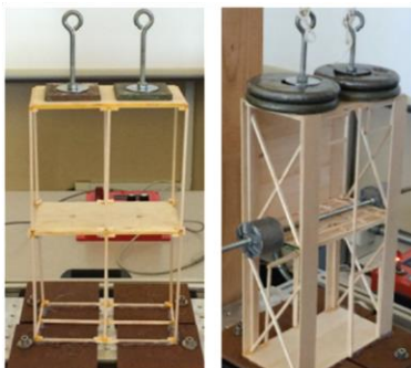
Figure 3. Shear Wall Design Demonstration: Structure with (Right) and without (Left) Shear Walls
