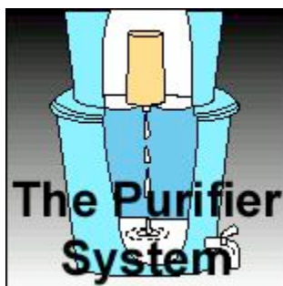
Figure 1: The Purifier water treatment system uses silver impregnated ceramics to provide safe drinking water ( http://www.purifier.com.np ).
