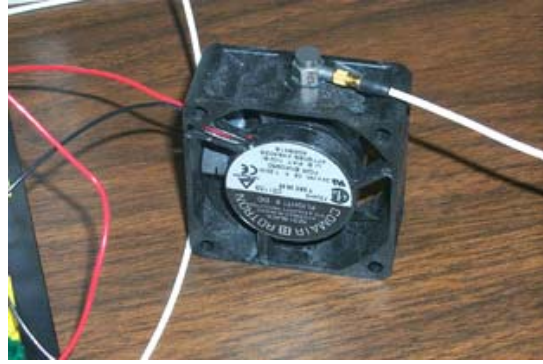
Figure 2: Motor accelerometer set-up.
