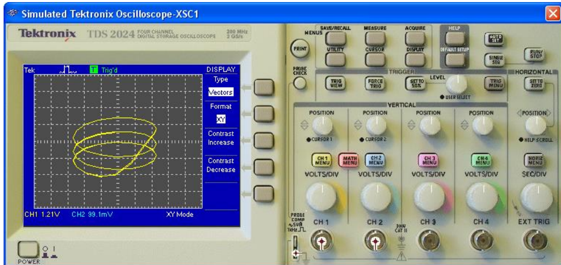
Fig. 3(c). Phase portrait of V_{in} versus V_R
