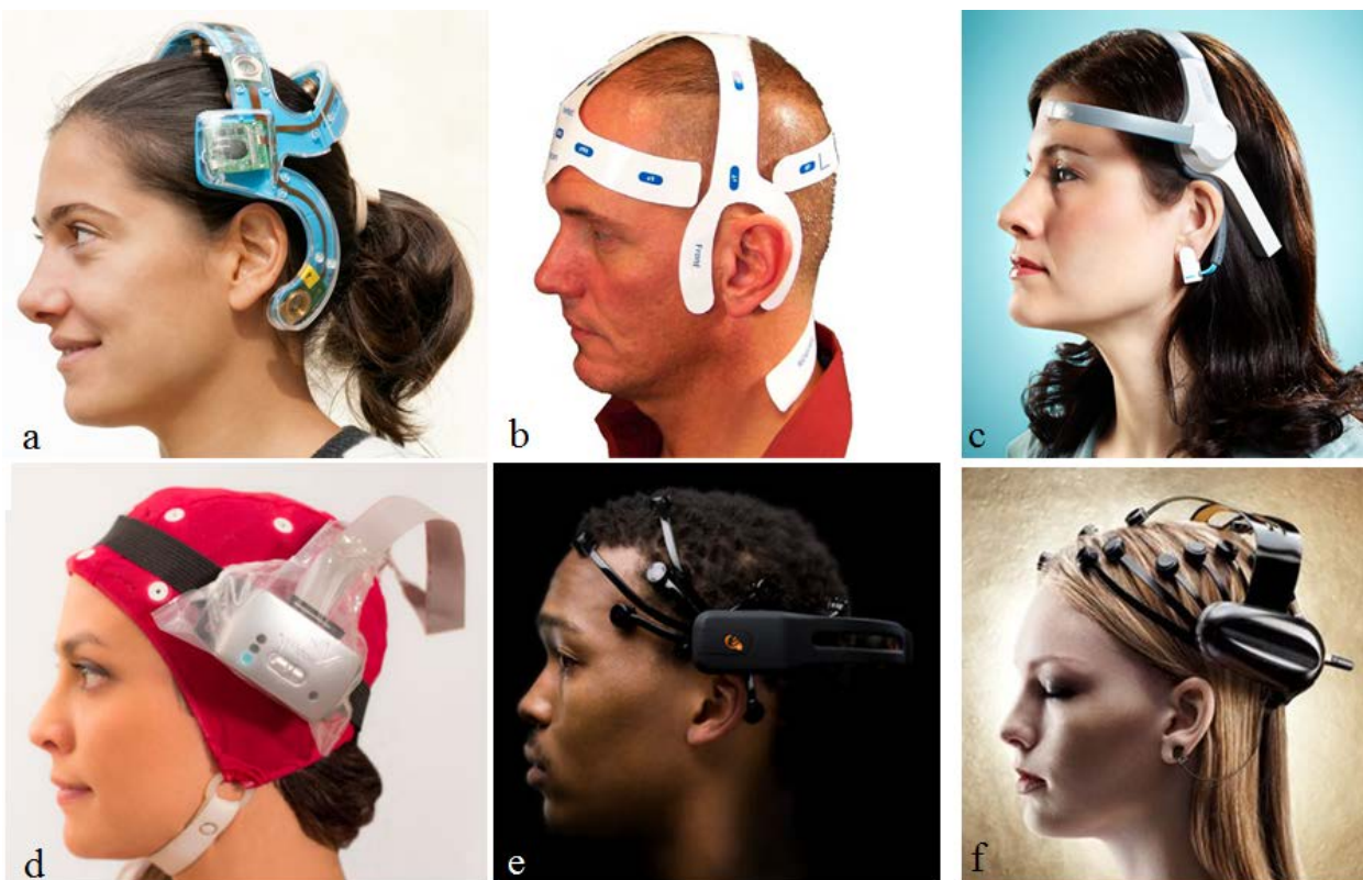
Fig. 4: Some of the commercially available EEG measuring devices and electrode setup. a IMEC Wireless EEG b . StatNet Disposable EEG c . Neurosky Mindwave d . MicroEEG e . Emotiv f . NeuroFocus
