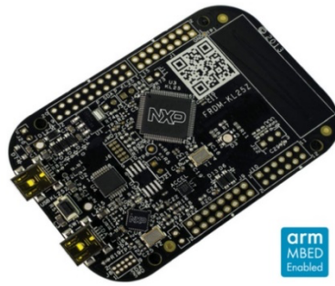
Figure 2 FRDM-KL25Z development board by NXP. This is an open source hardware board with Arduino compatibility
