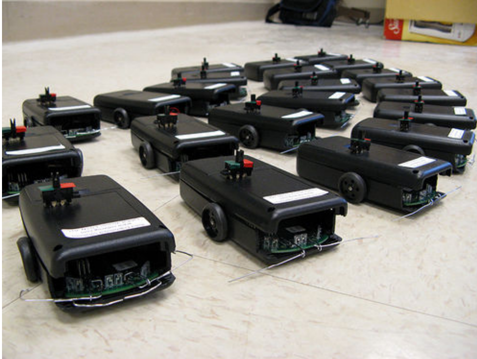
Figure 1. A swarm of 20 LabRats, constructed by students enrolled in the Introduction to Robotics Course at the Missouri University of Science and Technology.
