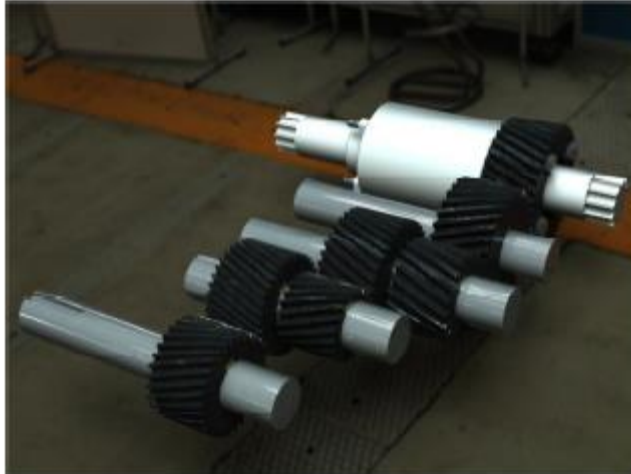
Figure 10: 3D CAD view of the designed gear train.
