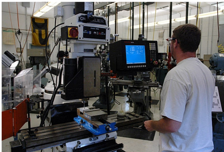
Figure 2: CNC vertical mill used for cutting flat layout.
