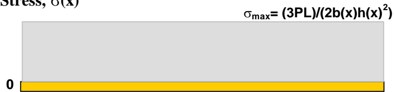
Figure 4: A simply supported beam with a constant flexural bending stress, \sigma(x) , for a beam that has variable cross-section along x .
