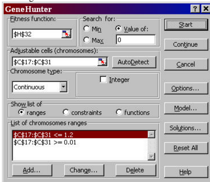
Figure 10: Genetic algorithm set-up screen using Ward System Group's GeneHunter™ to produce values of beam width, b(x) , for a constant stress beam with cell H32 representing the sum of the deltas
