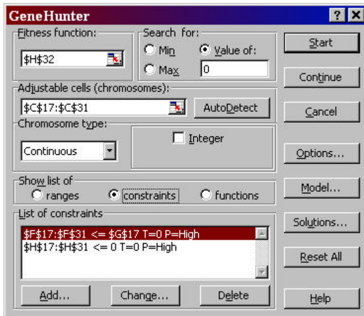
Figure 11: Genetic algorithms method with constraints for stress ( \leq G17 ) and deltas ( \leq 0 )
