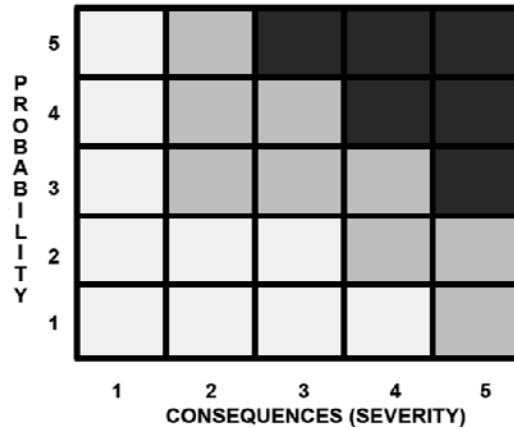
Figure 8: Risk matrix. Plotting the consequence and probability values for each risk item yields a risk level of low (light gray), medium (med. gray) or high (dark gray).
