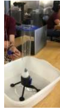
Figure 10. Rain gauge to control irrigation system rate.
