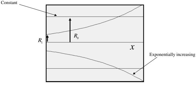
FIGURE 4 -CONSTANT AND EXPONENTIALLY VARYING SHAFTS
