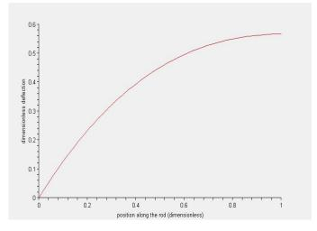
FIGURE 5 - ROD DEFLECTION - INCREASING AREA CASE
