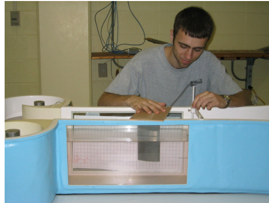
(b) Water Tunnel Test Section
