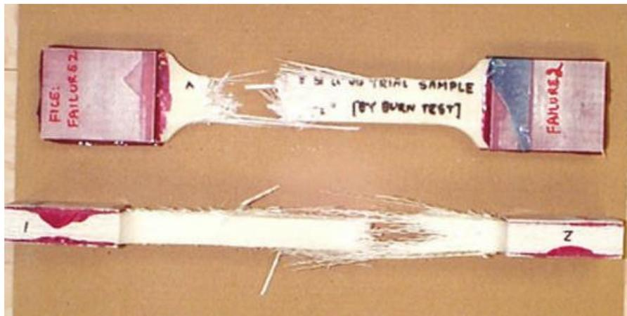
Figure 7 Composite coupons failed in tension test
