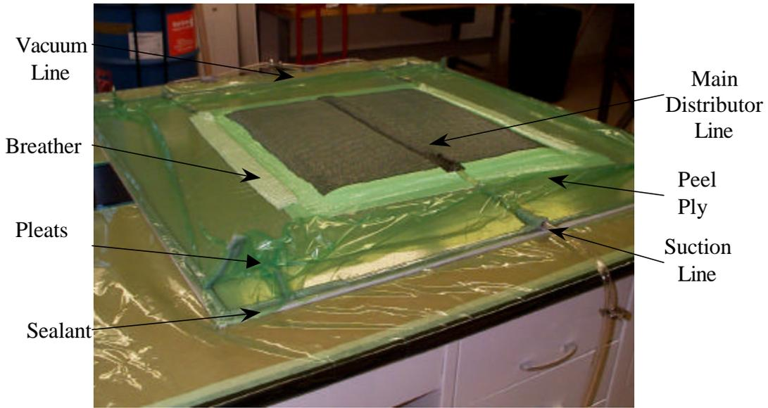
Figure 1 VARIM fabrication setup photograph
