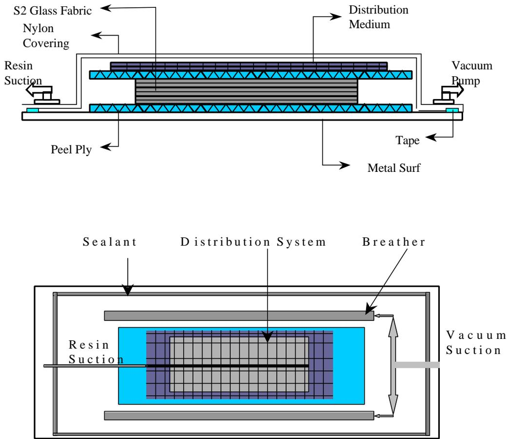
Figure 2 VARIM fabrication schematic
