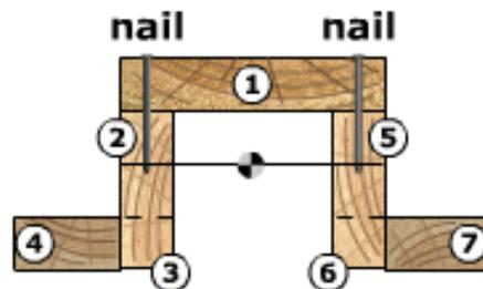
6. The sketch shows two cross-sectional configurations: Beam A and Beam B. Both Beam A and Beam B have the same shear force  $V$ , the same moment of inertia  $I$ , and the same nails. The nails in Beam A are spaced at 5-inch intervals along the beam span. For Beam B, the nail spacing will be:
