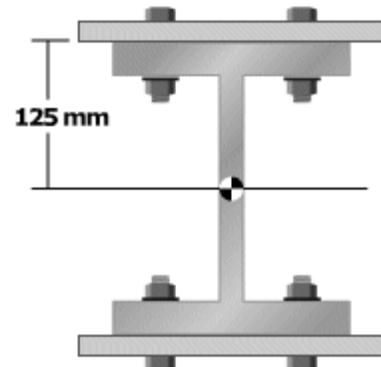
8. If the cross-sectional area of each bolt is 200 mm<sup>2</sup> and the allowable shear stress is 60 MPa for the bolts, how much shear flow  $q$  can the beam withstand?
