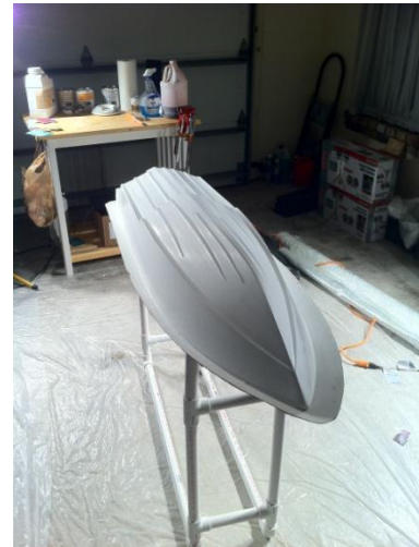
Figure 3: Hull fabrication after gel coat has been applied.
