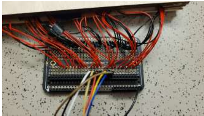
Fig 7b: Transducer wires soldered to PCB
