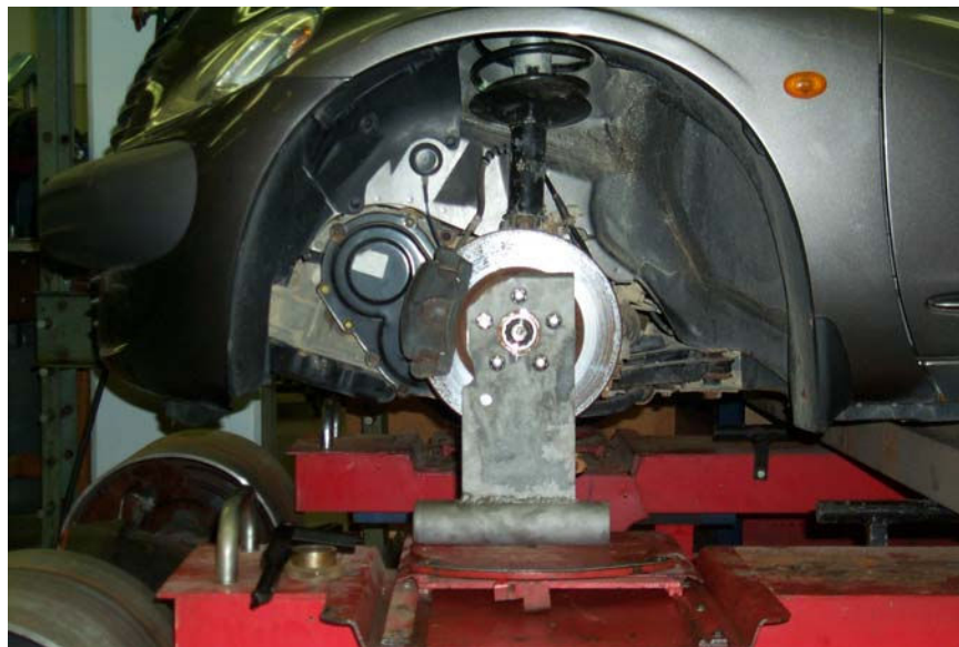
Figure 1. Steel foot in place of wheel to facilitate measurement
