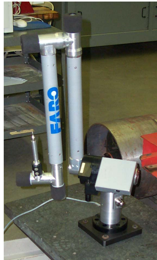
Figure 2. Bolt heads used to set up reference frame Figure 3. FARO arm for measurement
