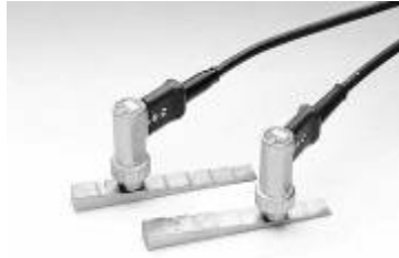
Fig. 2. Calibration of the flaw detectors using a straight-beam probe.
