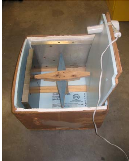
Figure 3. Photograph of Insulated Wood Box used to Heat the Aluminum Plates
