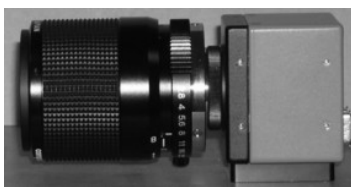
Figure 2. A CCD camera (DMK 21F04 by TheImagingSource) and a telecentric lens (TEC-M55 by Computar).
