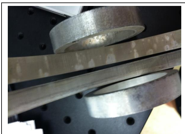
Figure 4 – Aluminum electrodes after use in salt water
