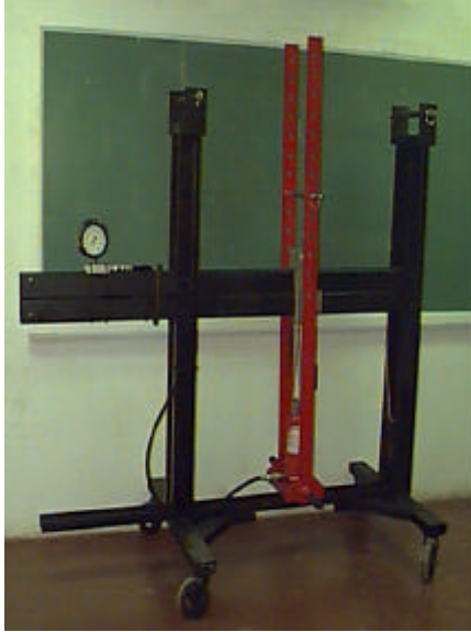
Figure E2 - Picture of truss testing device.
