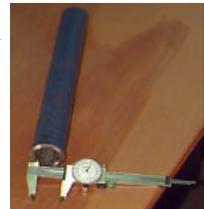
Figure 13 - Drill pipe measurement.
