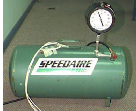
Figure 7 - Pressure vessel with pressure gage and strain gage.
