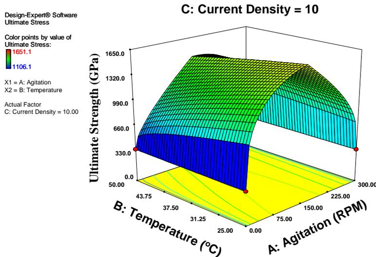
Figure 5. Young modulus (GPa) 3D surface plot as function of agitation and temperature; current density is fixed at 10.0 mA/cm<sup>2</sup>.
