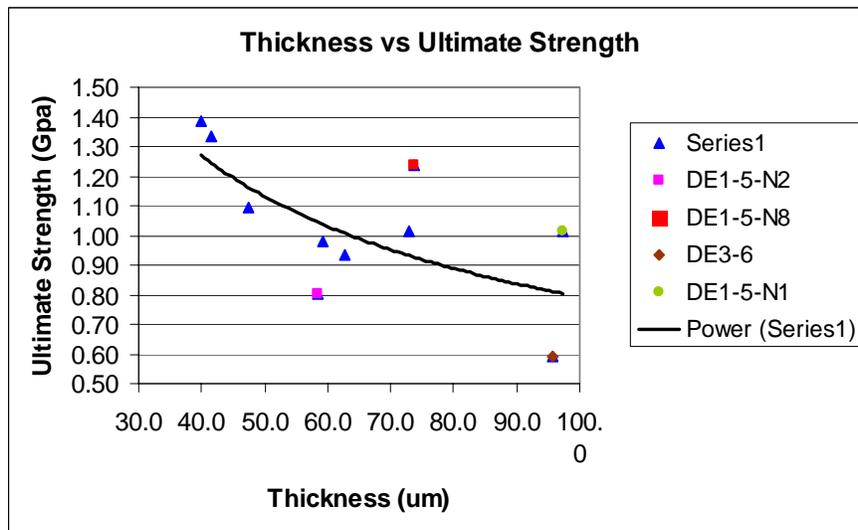
Figure 3. Plot showing ultimate strength ( $\sigma_{ult}$ ) as a function of specimen thickness.
