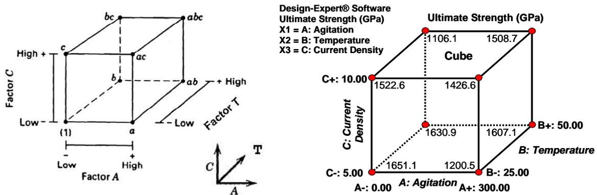
Figure 4. (Left): Treatment combinations in the  $2^3$  design. (Right): Treatment combinations in the  $2^3$  design for ultimate strength ( $\sigma_{ult}$ ); with measured  $\sigma_{ult}$  values (in GPa).
