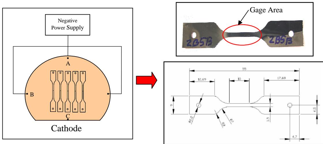
Figure 3. (Left) A Si wafer containing five electrodeposited Ni<sub>80</sub>-Fe<sub>20</sub> test specimens; and (Right) an actual Ni<sub>80</sub>-Fe<sub>20</sub> test specimen (top) with schematic drawing (bottom) of a reference ASTM dog-bone shape Ni<sub>80</sub>-Fe<sub>20</sub> test specimen depicting dimensions (in millimeters).
