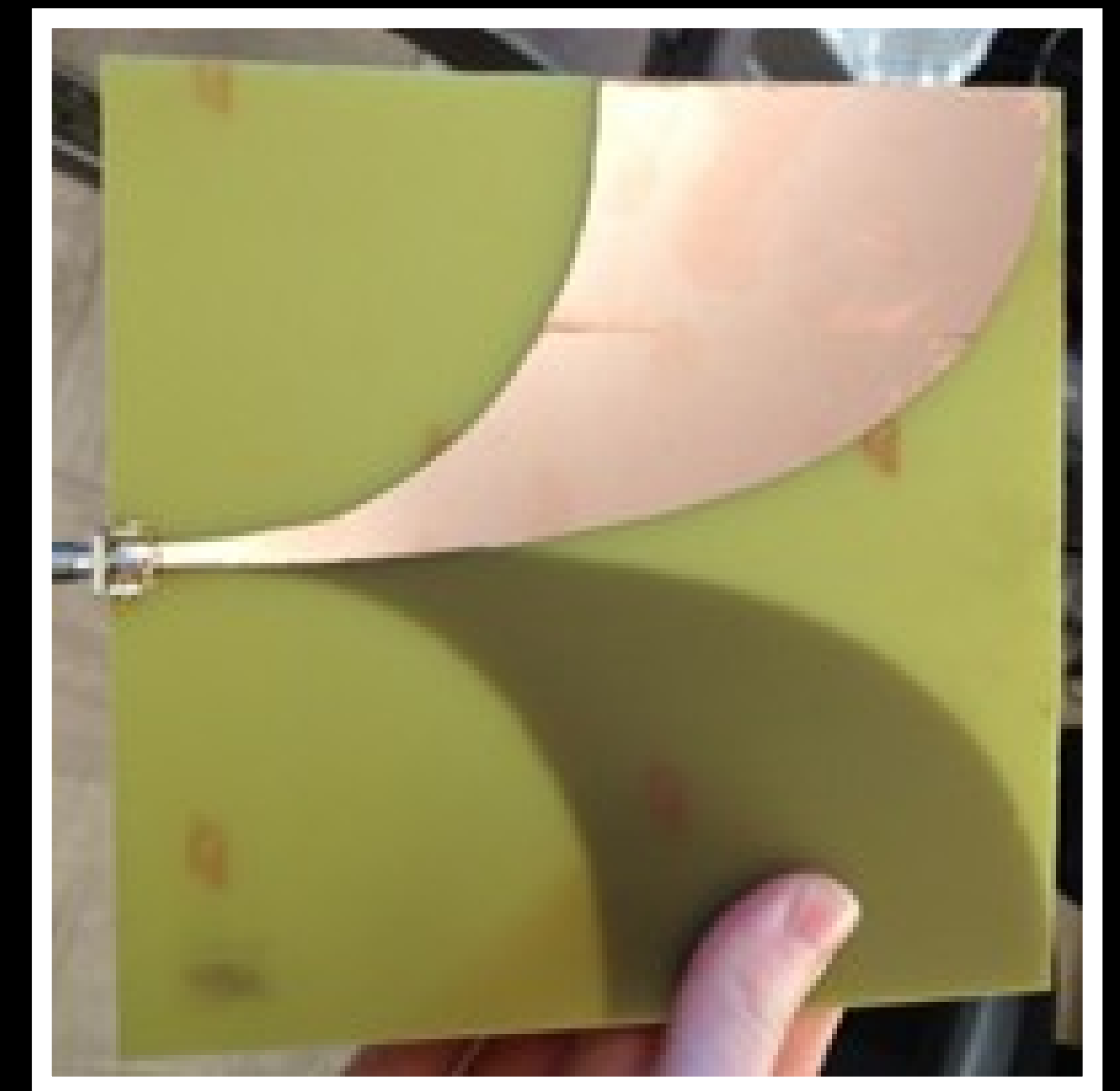
Completed Vivaldi prototype antenna
