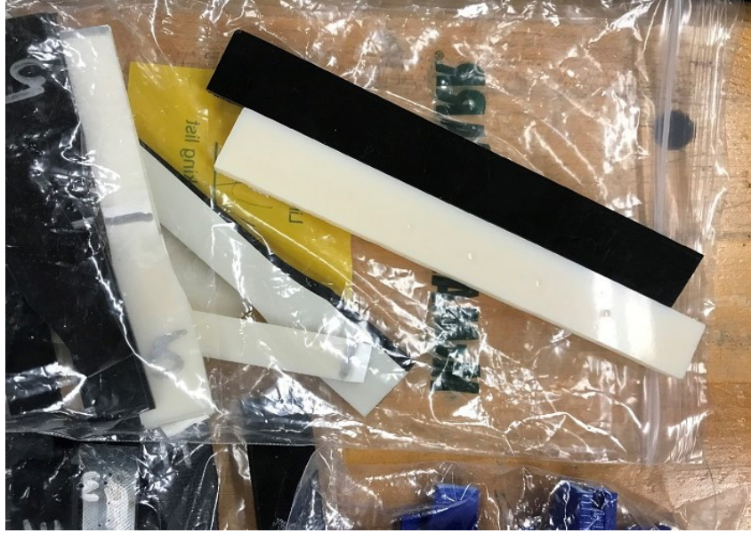
Figure 2: CNC machined cut-to-size specimens for hardness test
