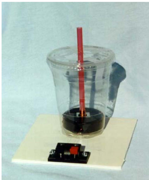
Figure 3: Electrodynamic Loudspeaker Constructed from a Plastic Cup.
