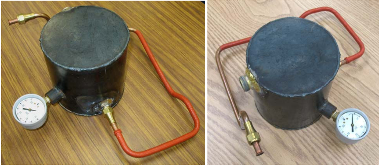
Figure 9. Two views of the exhaust tube flow calibration apparatus
