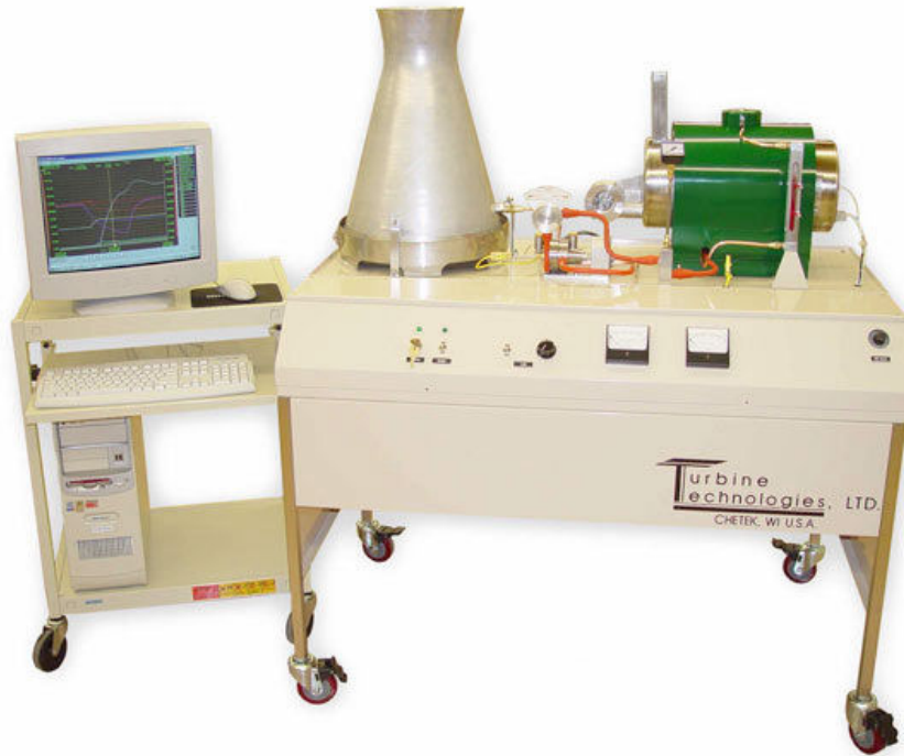
Figure 1: The Rankine Cycler. Note that the newer models include a USB port data acquisition system and laptop computer that is mounted to the tabletop 2 .
