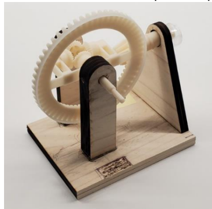
(f) Laser cut base and 3D printed components
