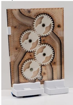
(e) Laser cut wooden frame with 3D printed components
