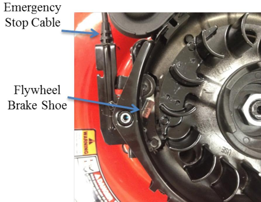
Figure 2: the emergency cable connects to the flywheel cowling and supports the flywheel brake shoe. There is also an electrical connection that stops the spark plug from firing when the handle is released.
