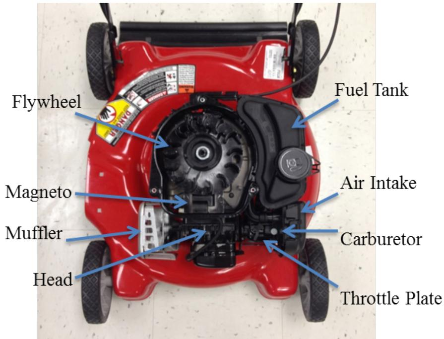
Figure 1: top view with cowling removed
