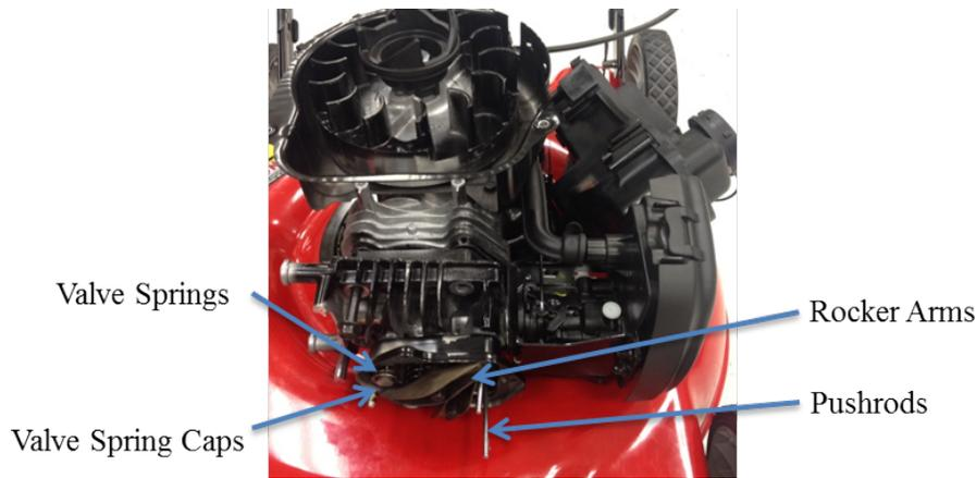
Figure 4: valve springs, rocker arms, and pushrods
