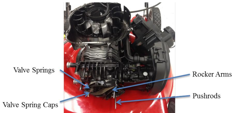
Figure 11: valve springs, rocker arms, and pushrods
