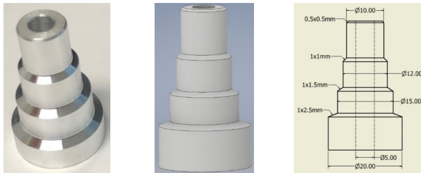
Fig. 12 Support, 3D model, and engineering drawing
