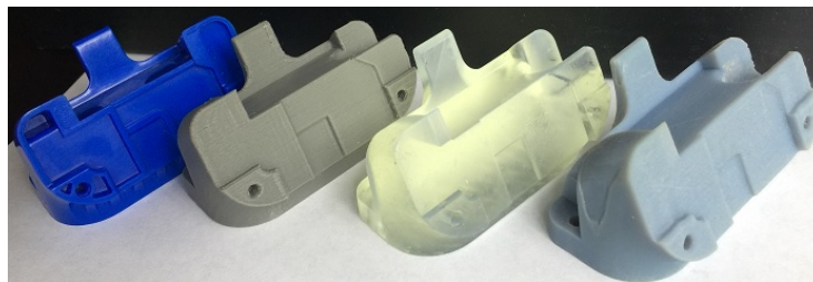
Fig. 3 Original and 3D printed Bulkhead (from left: original, FDM, SLA, and MJ)
