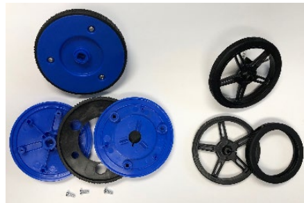
Fig. 4 Original (left) and Pololu 60x8mm (right) wheel-tire assembly
