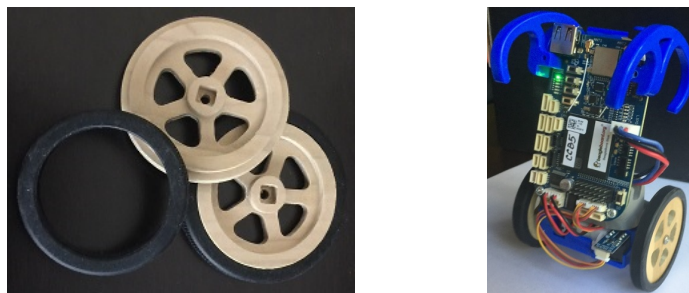
Fig. 7 CNC milled redesigned wheel (left) & a MIP with the new wheels (right)
