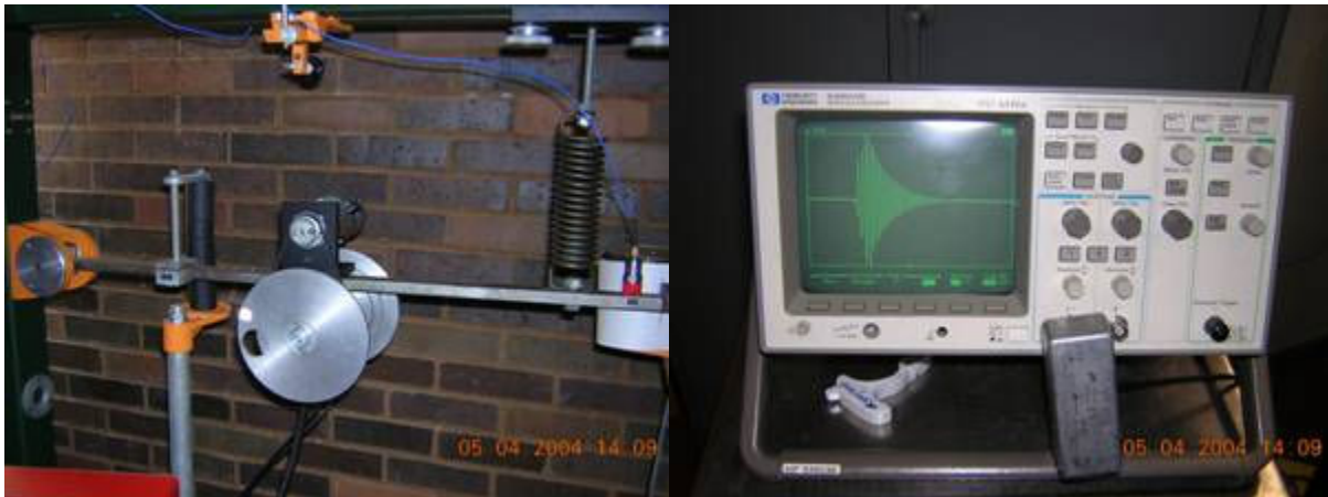
Figure 2 The designed mechanical system with accelerometer and its free vibration response
