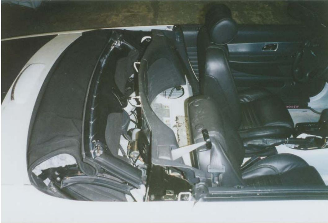
**Figure 5. Thunderbird Prototype Vehicle Showing Stowed Convertible Top**
