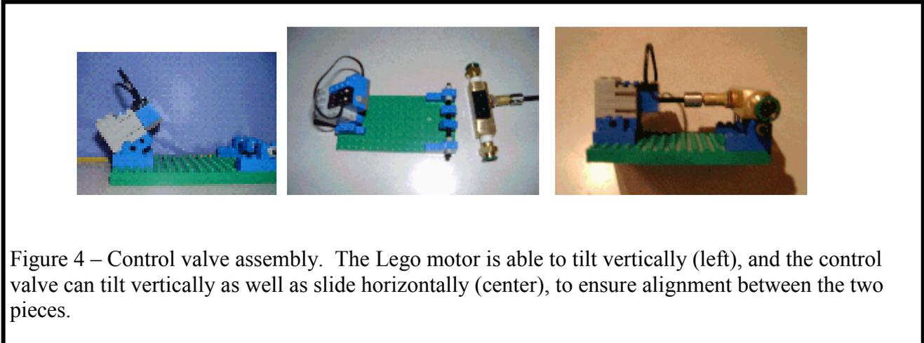
Figure 4 – Control valve assembly. The Lego motor is able to tilt vertically (left), and the control valve can tilt vertically as well as slide horizontally (center), to ensure alignment between the two pieces.
