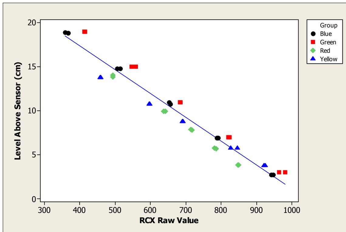
**Figure 1:** Student generated calibration curves for the new pressure sensor based on the Honeywell Micro-switch pressure sensor and a Techno-stuff four-wire interface to the RCX brick.
