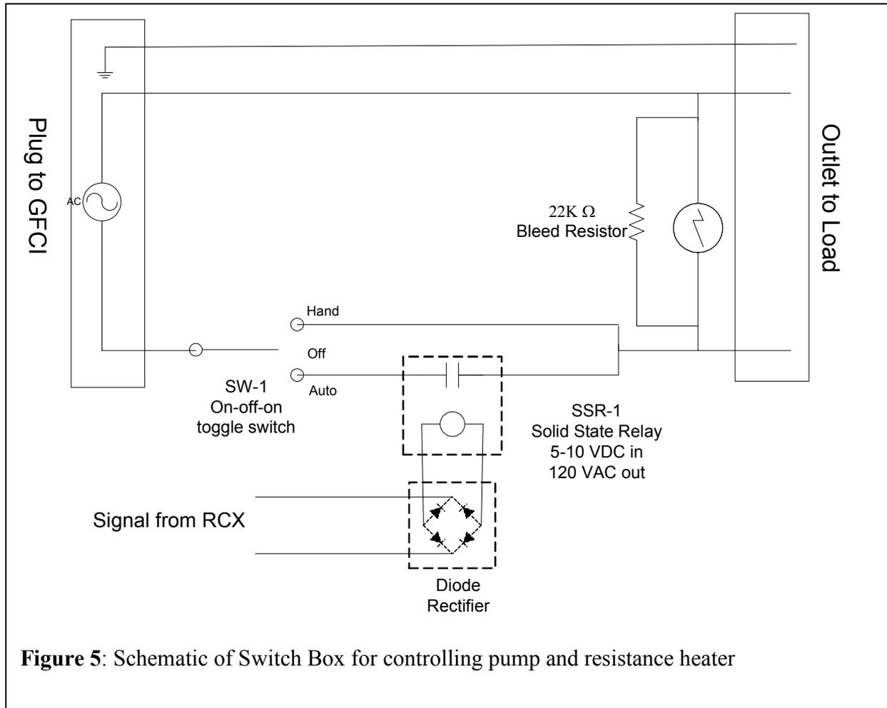
**Figure 5:** Schematic of Switch Box for controlling pump and resistance heater
