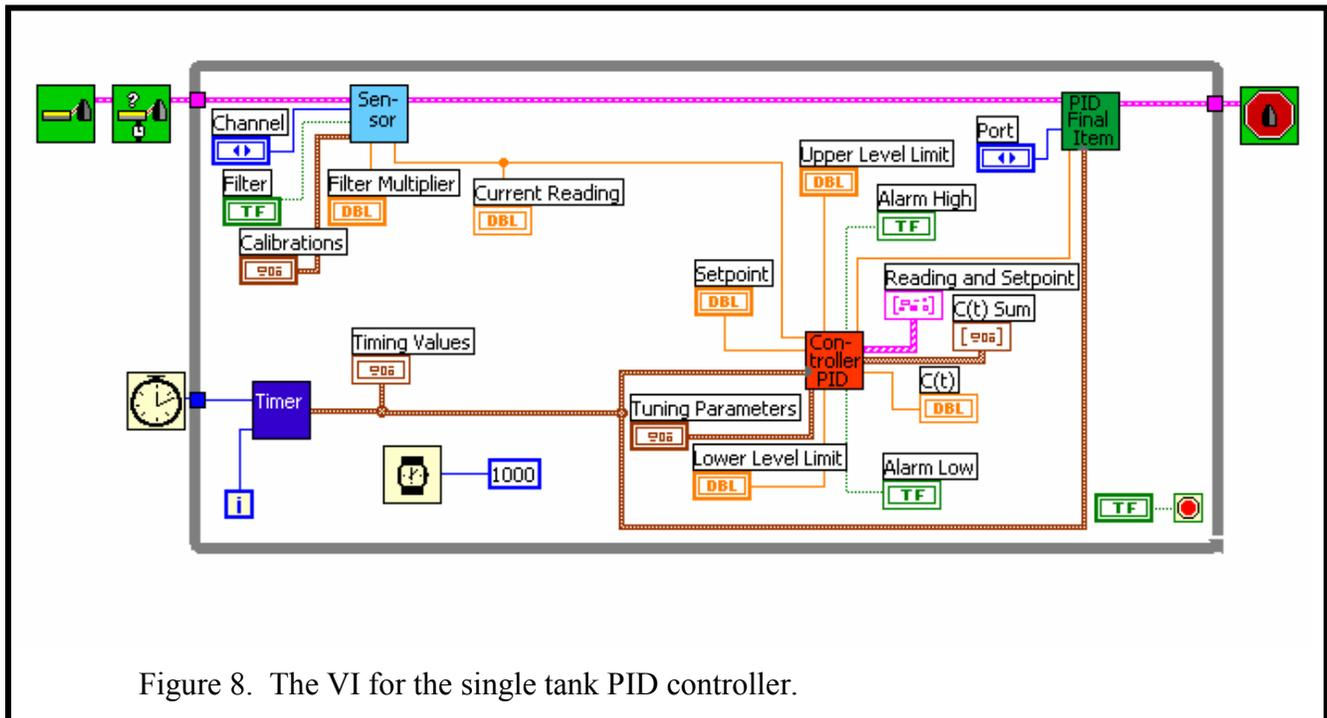
Figure 8. The VI for the single tank PID controller.
