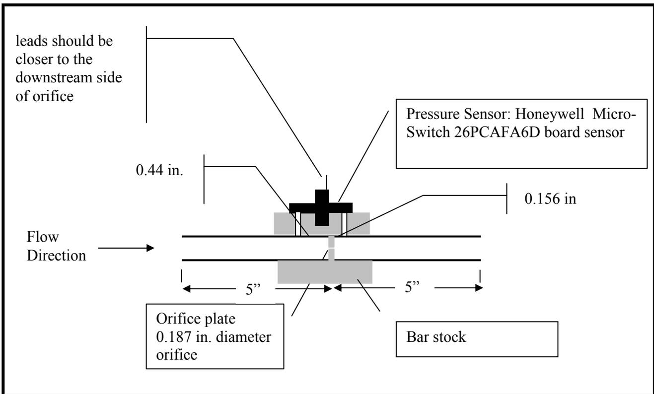
Figure 2. Diagram of the orifice meter.
