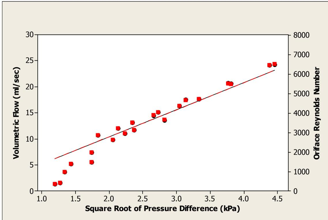
Figure 3: Calibration curve for orifice meter.
