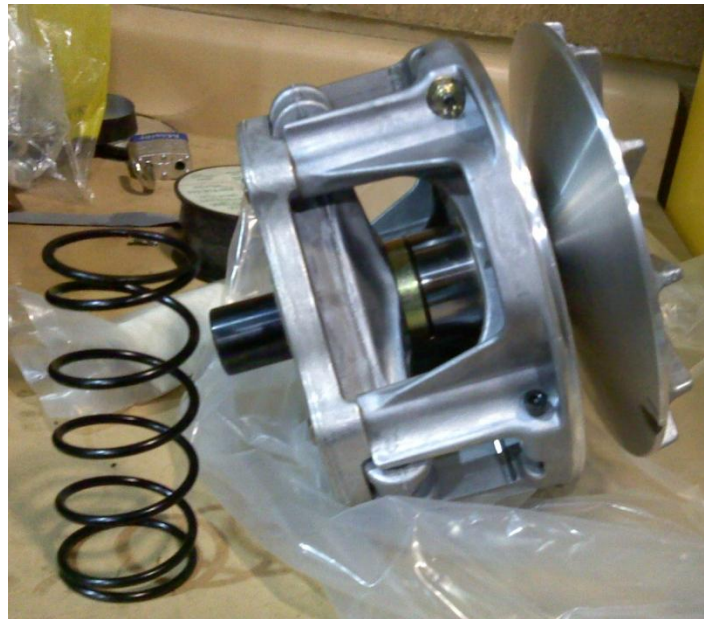
Figure 4 Polaris P90 CVT used on our 2 nd year vehicle
