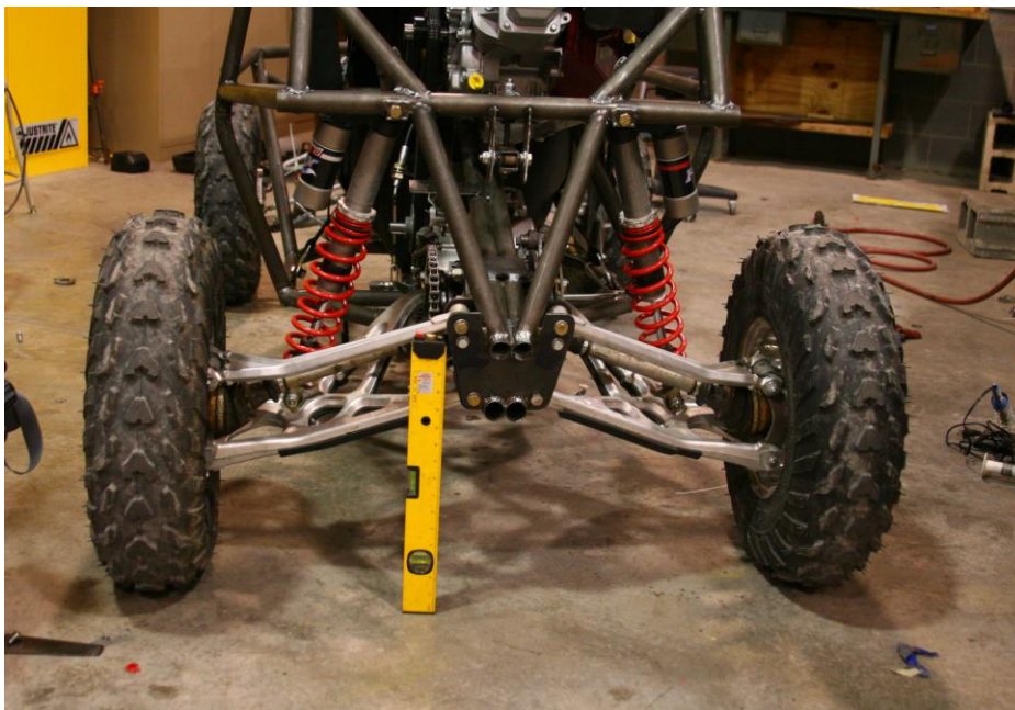
Figure 1 Our first year vehicle with a Polaris ATV suspension (center clearance of 12")
