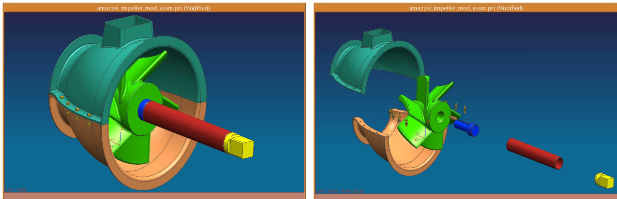
Figure 6 – impeller assembly (with exploded view)
