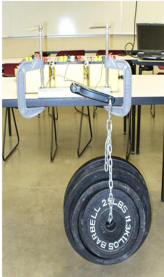
Figure 2. Static testing of the torque sensing crank arm.
