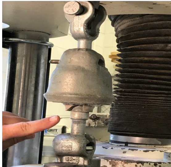
Figure 2: Failure and point of fracture is observed in a practice run of testing.
