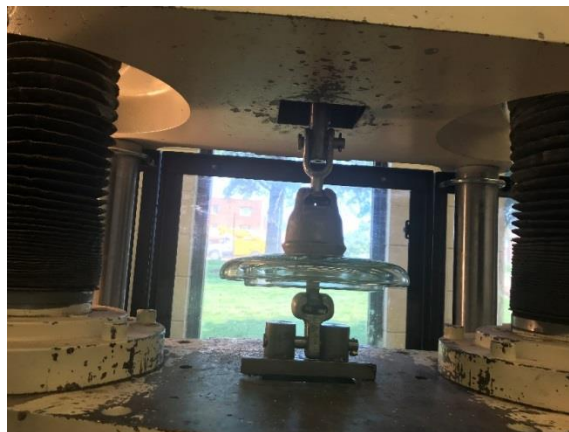
Figure 1: Glass insulator loaded in the Tinius Olsen Tensile Testing Machine
