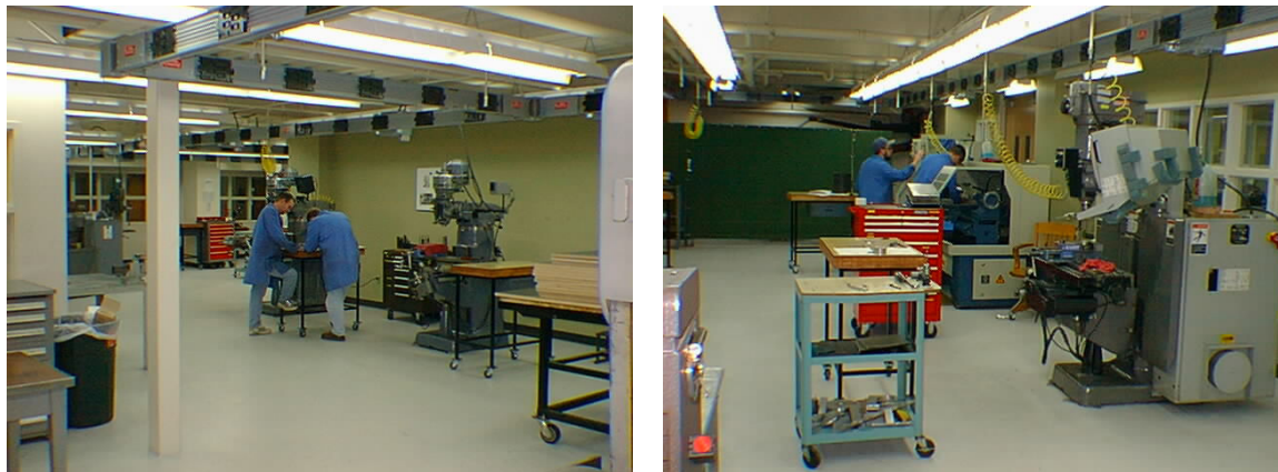
Figure 1. Engineering Shop: Manual Mills (left), 2-axis CNC mill and CNC lathe (right)
